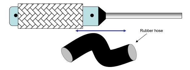
C. Install the rubber hose you want to be protected on the metallic mandrel. It changes temporarily the shape of the hose and makes the braided sleeve installation easier.
