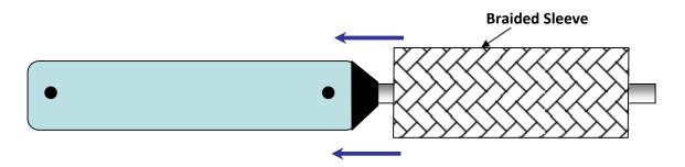
B. The sleeve has to cover completely the cartridge. Make the cartridge move alongside the mandrel to lubricate it.
