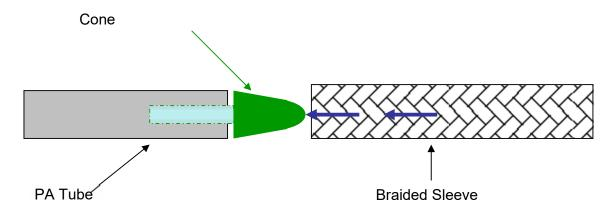
The cone at the end of the PA tube makes the installation easier
