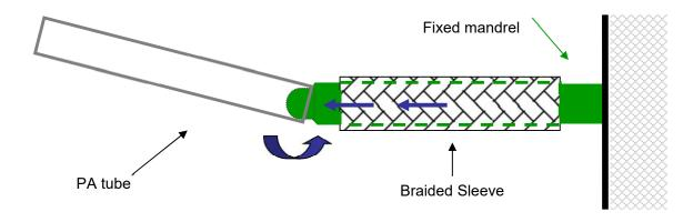
C. Install the braided sleeve on the PA tube by pulling it
