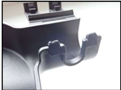
The figure 8 Short shot/not completely moulded
