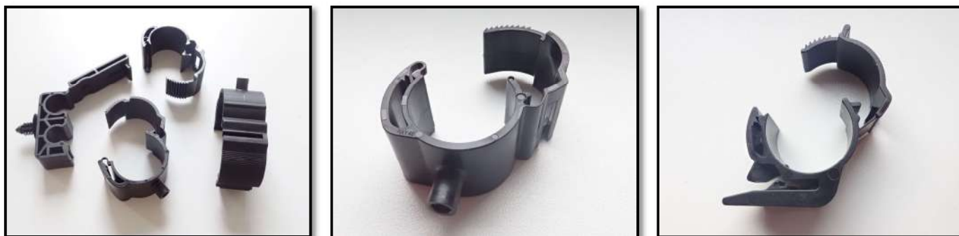
The figure 2 Parts with film hinges
