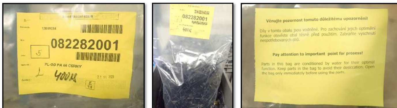
The figure 1 Water conditioned parts
