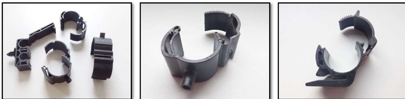
The figure 2 Parts with film hinges
