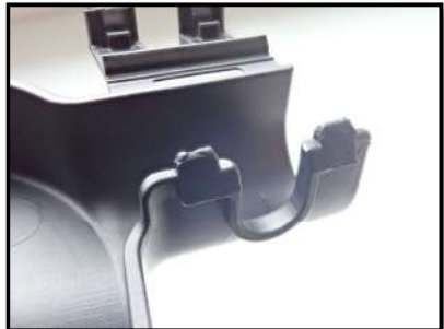
The figure 8 Short shot/not completely moulded
