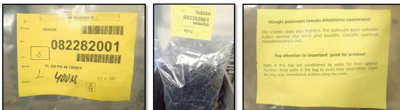
The figure 1 Water conditioned parts
