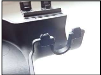
The figure 8 Short shot/not completely moulded
