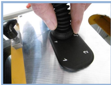
Picture 4: Assembly of cover at hook 3
