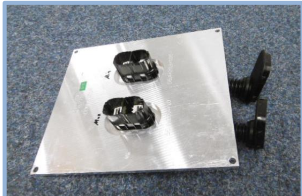
Picture 3: Sheet metal with grommet, dry side
