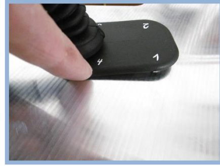
Picture 5: Assembly of cover at hook 4
