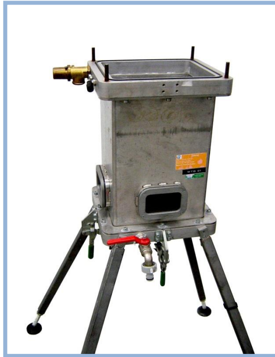
Picture 1: ESD Water Test Equipment
