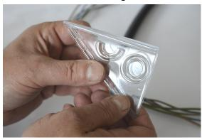
B. Insert the cables in the mounting tool.
